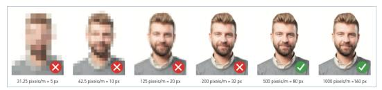
5. Select such a focal length of the camera's lenses that provides the required pixel density at a predetermined distance to the recognition objects. The picture below demonstrates how to calculate the focal length subject to the distance between the camera and recognition objects. Estimating the focal length for a particular camera requires either calculators or a methodology provided by the camera manufacturer.
