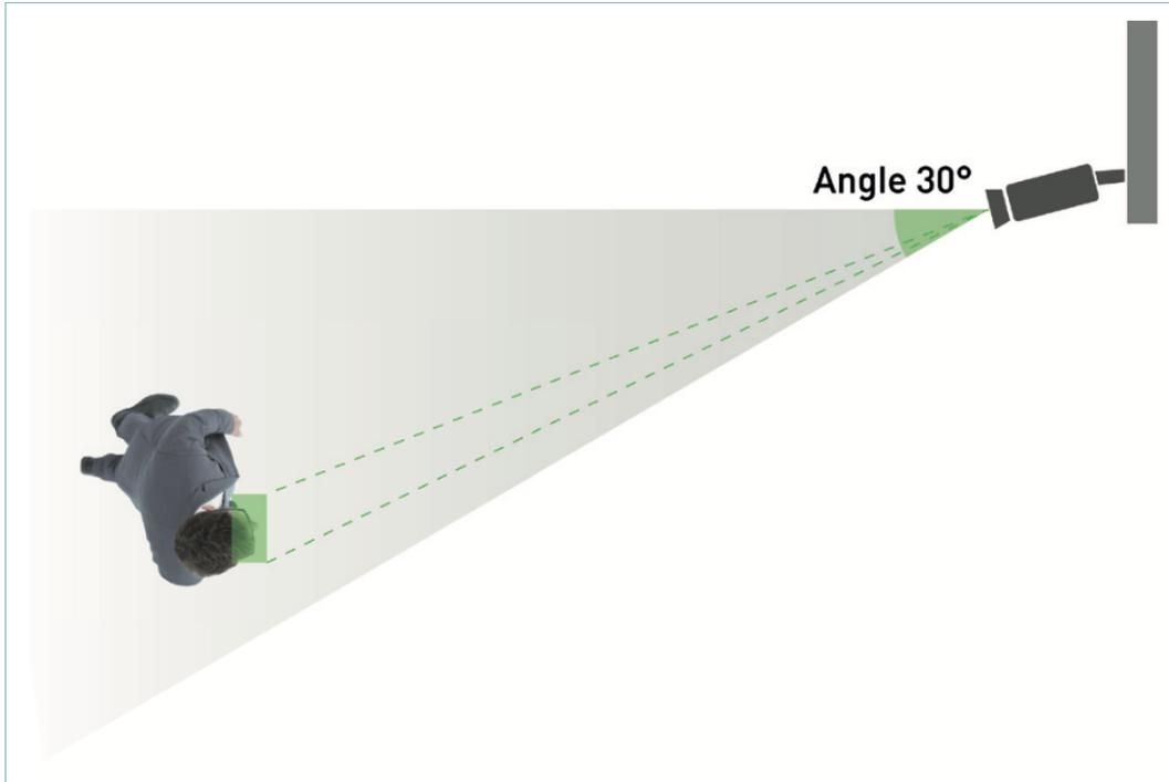
4. The minimum pixel density required for identification is 500 pixels/m (roughly corresponds to a face width of 80 pixels).
