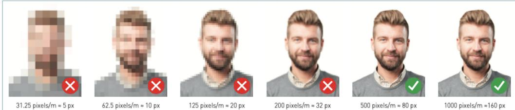
5. Select such a focal length of the camera's lenses that provides the required pixel density at a predetermined distance to the recognition objects. The picture below demonstrates how to calculate the focal length subject to the distance between the camera and recognition objects. Estimating the focal length for a particular camera requires either calculators or a methodology provided by the camera manufacturer.
